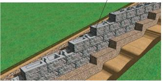
\_\_\_ Capping Units Attached with Concrete Adhesive
