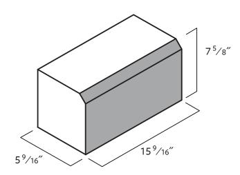
1F/1E Chamfer End Solid Only face and angled unit will be ground
