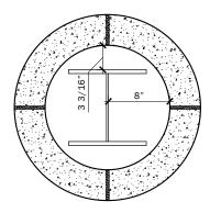
Steel Column - Minimum size W10x49 with minimum air space from web to block of 8 in. and from flange to block of 3 3/16 in. See above illustration.
